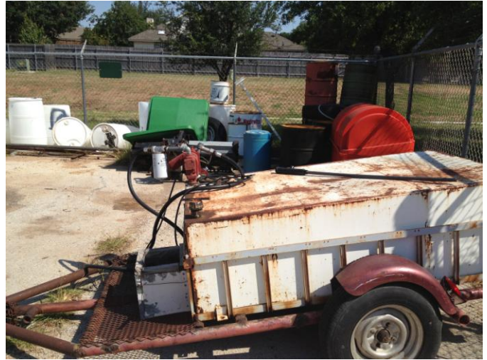
250-gallon portable diesel AST at the Physical Resources Building
